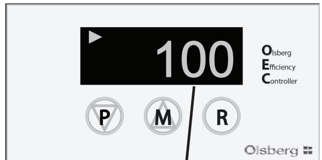
Indicates combustion air slide valve position is 100% open
